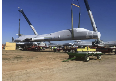
B-1B Lancer tail number 85-0022 is lifted and placed on ballbed trailers for its journey to Wichita, Kan., on April 24, 2020. The National Institute for Aviation Research at Wichita State University planned to scan every part of the aircraft to create a digital twin for research. (Clay Mayer/U.S. Air Force)
